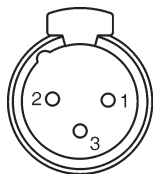
DMX - output XLR mounting-sockets (rear view):
