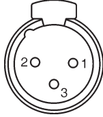
DMX - output XLR mounting-sockets (rear view):
