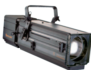
EVO 25 DH ZS 2500 W/HTI, G 22 Adjustable beam from 8° to 16° Shaping shutters and sliding guides for gobo holder or iris Internal DMX dimmer 270x314x1230 mm - 36 Kg Ballast: 270x299x406 mm - 33.3 Kg
