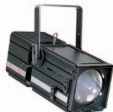
FI 25 ZW 2000/2500 W, G 22 Adjustable beam from 17° to 36° Shaping shutters and sliding guides for gobo holder or iris 270x294x800 mm - 21.3 Kg
