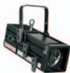
FI 05 ZS 300/500/650 W, GY 9.5 Adjustable beam from 14° to 33° Shaping shutters and sliding guides for gobo holder or iris 150x150x497 mm - 4.8 Kg
