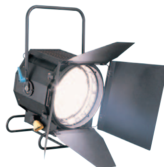
FR 25 MSR Metal halide lamp MSR 2500 W G 38 Adjustable beam from 7° to 70° Lens ø 300 mm 470x445x395 mm - 25 Kg Power supply: 270x299x406 mm - 33.3 Kg
