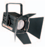
AR 05 300/500/650 W, GY 9.5 Adjustable beam from 7° to 62° 150x150x273 mm - 2.9 Kg
