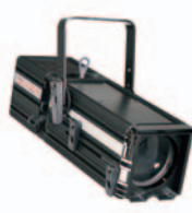
FI 12 ZS 1000/1200 W, GX 9.5 Adjustable beam from 13° to 35° Shaping shutters and sliding guides for gobo holder or iris 200x200x726 mm - 9.8 Kg
