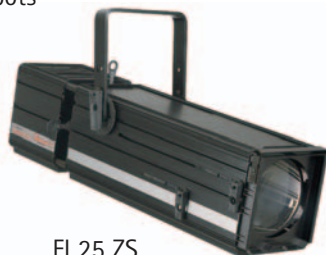
FI 25 ZS 2000/2500 W, G 22 Adjustable beam from 9° to 25° Shaping shutters and sliding guides for gobo holder or iris 270x294x1147 mm - 25.1 Kg
