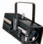
FI 12 ZW 1000/1200 W, GX 9.5 Adjustable beam from 24° to 50° Shaping shutters and sliding guides for gobo holder or iris 200x200x578 mm - 9.1 Kg
