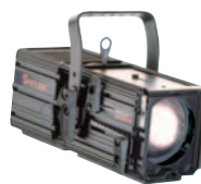
EVO 12 DC ZW 1200 W/HTI/SA, GY 22 Adjustable beam from 23° to 36° Shaping shutters and sliding guides for gobo holder or iris Internal DMX dimmer 200x224x578 mm - 14.9 Kg Ballast: 200x204x256 mm - 14.8 Kg
