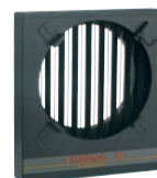
FR 25 MSR Metal halide lamp MSR 2500 W G 38 Adjustable beam from 7° to 70° Lens ø 300 mm 470x445x395 mm - 25 Kg Power supply: 270x299x406 mm - 33.3 Kg
