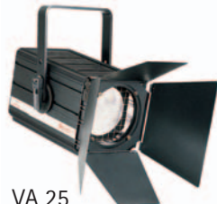
VA 25 2000/2500 W, G 22 Adjustable beam from 4° to 66° 270x293x543 mm - 13.1 Kg
