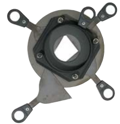
4 removable shaping shutters mounted between plates specially treated with an anti-abrasive surface and locked by long-extension springs to allow the shutters to be moved smoothly and precisely
