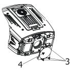
**4.** Place the long (short) throw optic module (5) instead of the module of the glass cover (4) and secure it by the 3 quarter-turn fasteners (6).
