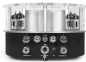
Insert the power cord into the rear panel of the amplifier. Select the voltage on the adapter to your local voltage 110V or 230V. Connect the power cord to the adapter and plug the other end into an AC wall jack
