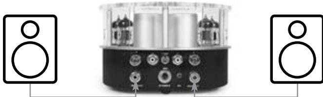
Connect the amplifier to the speakers with enclosed audio source wires and make sure the L and R connection are correct. Select your speakers with impedance greater than 8 ohm, otherwise you may damage the amplifier system.
