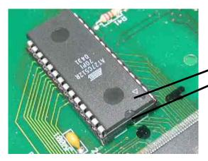
The recessed groove of the EPROM must be aligned with the marking (white line) on the PCB.
