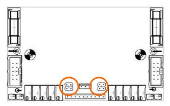
Some software packages require inverting of the Y-channel. The driver board contains an inverting circuit on every channel. To invert one channel, you need to remove the head cover of the Sniper<sup>45</sup>.
