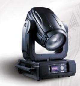
The ColorWash 700E AT is the first Wash fixture using the MSR GOLD 700 FastFit lamp in the Robe range. This powerful moving head offers a full CMY + CTO colour mixing system, a colour wheel with 7 replaceable "SLOT&LOCK" dichroic filters, a rotating beam shaper and a linear zoom range of 6° - 45°.
