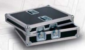
The Lid Set for REDWash/Flash  $3 \cdot 192$  was designed to separate double cases into two single cases. It is constructed from high-quality, water repellent 13mm thick plywood with exterior covered in black finish. It has a black finished exterior and features aluminium protected edges and tough steel corners.
