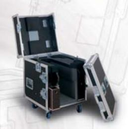
This case provides perfect protection for Robe's DigitalSpot 3000 DT in the touring and rental market. It is constructed from high-quality, water repellent 13mm thick plywood. It has a black finish exterior and features aluminium protected edges and tough steel corners. This single case is equipped with four metal recessed wheels for easy transport.
