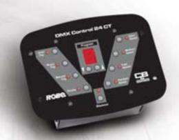
The DMX Control 24 CT is a compact DMX controller with 24 DMX control channels. The built-in microphone and audio input connector allows the program to be perfectly triggered to the beat of the music.
