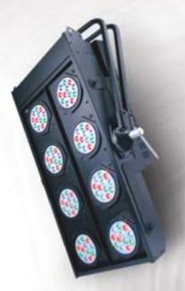
The REDBlinder 2.96 is fitted into the industry standard 8-lite casing and offers set and lighting designers all the options. REDBlinder is a LED version of the popular 8-lite Molefay, a staple of the rock "n" roll world, featuring 8 LED modules, each with 12 RGB K2 LEDs. Each four pairs of modules are separately controllable. This product is aimed at all stage lighting markets and television productions and for arenas and larger venues.
