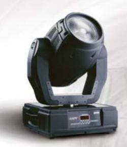
The ColorWash 575 AT is ideal for theatres, TV studios, medium sized stage applications and all applications requiring a "workhorse" 575 lamp. Offering full CMY, variable CTO, colour-wheel with 5 replaceable colours + open, combined dimmer/shutter and rotatable beam shaper, indexable 360° with continuous rotation. The standard zoom angle has a range of 12-34°, extendable with an optional lens to make 24-60°.
