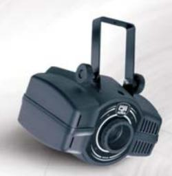
This effect projector is fully DMX controllable; projects tightly focussed flower effects and other graphic effects; offers original gobo designs; includes a parabolic mirror reflector that rotates in both directions; a combined gobo/colour wheel with 14 positions plus open; comes with a powerful 250W halogen lamp (1000hrs life); a strobe effect and 0-100% digital dimming; "auto-trigger" or "music-trigger" mode for full flexibility.
