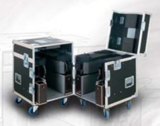
Designed to house two Robe REDWash/Flash 3•192 fixtures, this quality case is made from high-quality, water repellent 13mm thick plywood. Features include four heavy duty wheels for easy transport, reinforced carry handles on all four sides, butterfly style latches, steel ball corners and aluminium edge protection. Its exterior is covered with a black finish.
