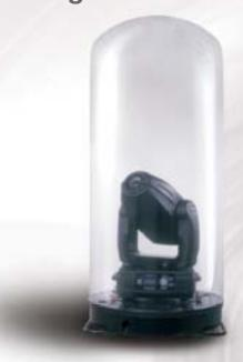
The Robe LightDome 1200 enables Robe 700/1200 AT Series fixtures to be used in outdoors installations in any type of weather. It is made from special transparent non-flamable PVC-P film, with an IP 43 protection factor. All the effects of the Robe fixture inside can be used as normal. Back-UPS holds the dome inflated for 8 minutes. It is to protect the plastic dome falling on the hot fixture.
