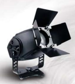
This fixture is a static colour changer with a fresnel lens. The ColorMix 250 AT is aimed at theatres, TV studios, stage lighting and interior and exterior architectural lighting. Features include CMY colour mixing plus an additional colour wheel, six dichroic colours and open, beam shaper, frost filter, dimmer shutter and an included barn door fitting for the front. The fixture can be floor standing or wall/ceiling mounted and offers the same functionality needed as the Wash 250 XT moving head.
