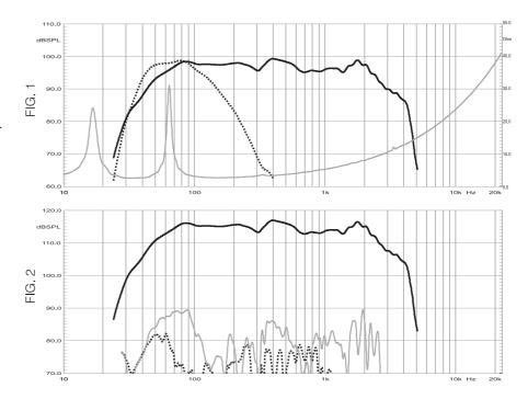
NOTES. 1.Frequency response: referred to 1 m; low end obtained through the use of near field techniques; one-third octave smoothed for correlation with human hearing. 5.Polars were acquired by placing the unit on a computer controlled turntable inside our anechoic chamber. Measurement distance was 4 m.
